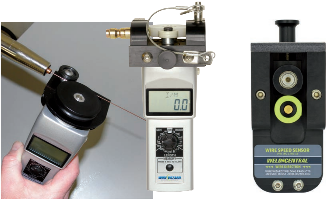
HHSS-12 obtaining measurement at the torch end
